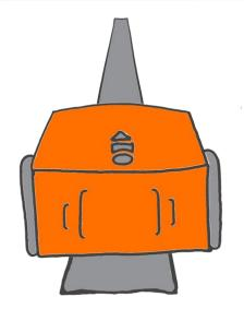
Edison uses a tracking sensor to see the difference between dark and light surfaces. Edison can use this sensor to follow a black line.
